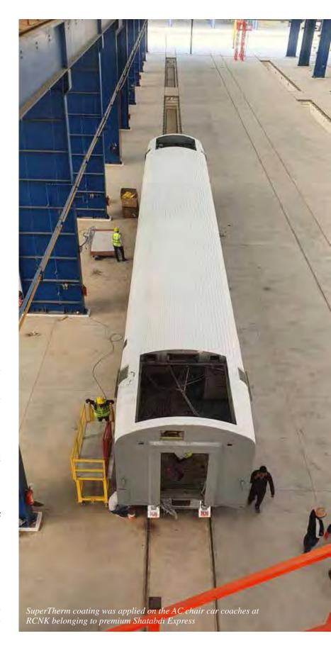
(NRLY). It was considered for applying on the roof shell exteriors of LHB air-conditioned coaches which were undergoing refurbishment at newly commissioned, state of the art Sonipat Rail Coach Naveenikaran Karkhana (RCNK) of Northern Railway. SuperTherm coating was applied on the AC chair car coaches belonging to premium Shatabdi Express (numbered 061179 NR LWSCZAC and 07902 NR LWACCN) at the workshop during thier periodic overhaul.
