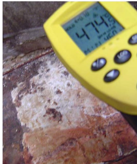
Surface temperature before HPC application: 474 C
