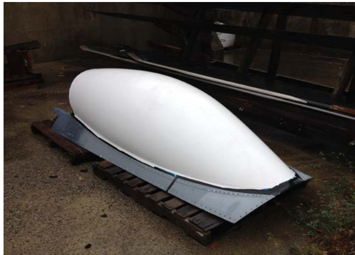
Figure 1: F16 Canopy with SPI coating applied
