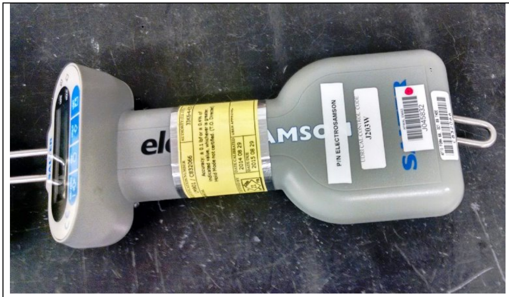
Figure 5: Salter Electrosamson Pull Tester
