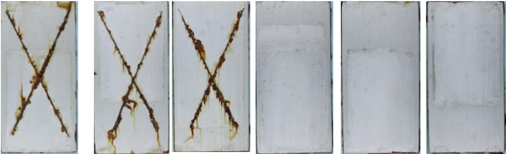
Figure 1. Rust Grip 1000 coupons' images after six weeks of exposure
