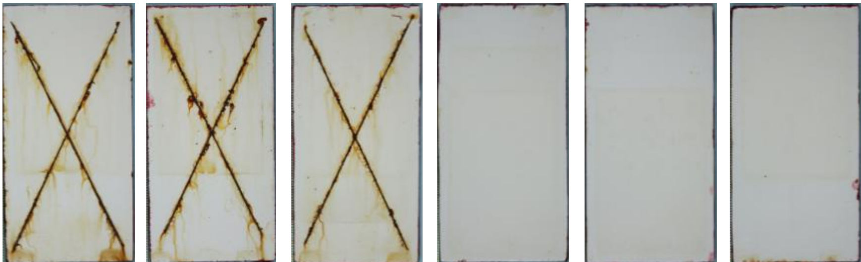
Figure 4. Moist Metal Grip coupons' images after six weeks of exposure
