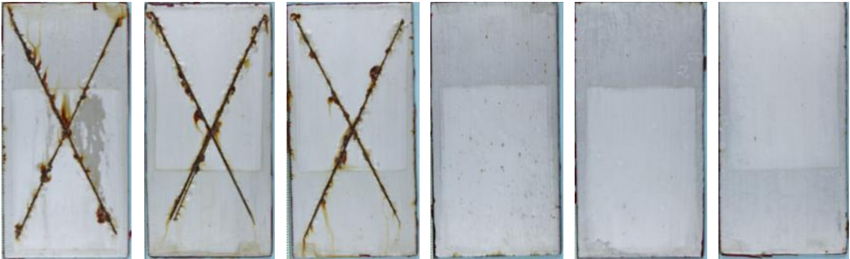
Figure 3. Rust Grip coupons' images after six weeks of exposure
