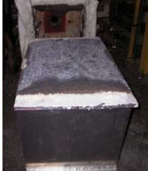
Figure 30 Char Formed Using Omega Fire™ Coating
