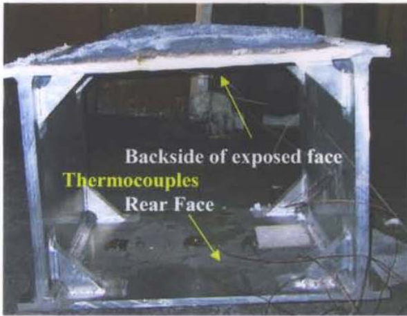
FIGURE 5. Aluminum Panel Undamaged with no warpage. Superior Products 2001F PFP Coating, Tested Using 2000°F Flame Temperature for 30 minutes. Note the lack of warpage.
