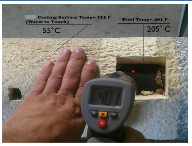
Inspection windows can be cut out of the coating film over weld joints for repeat non destructive inspection.
