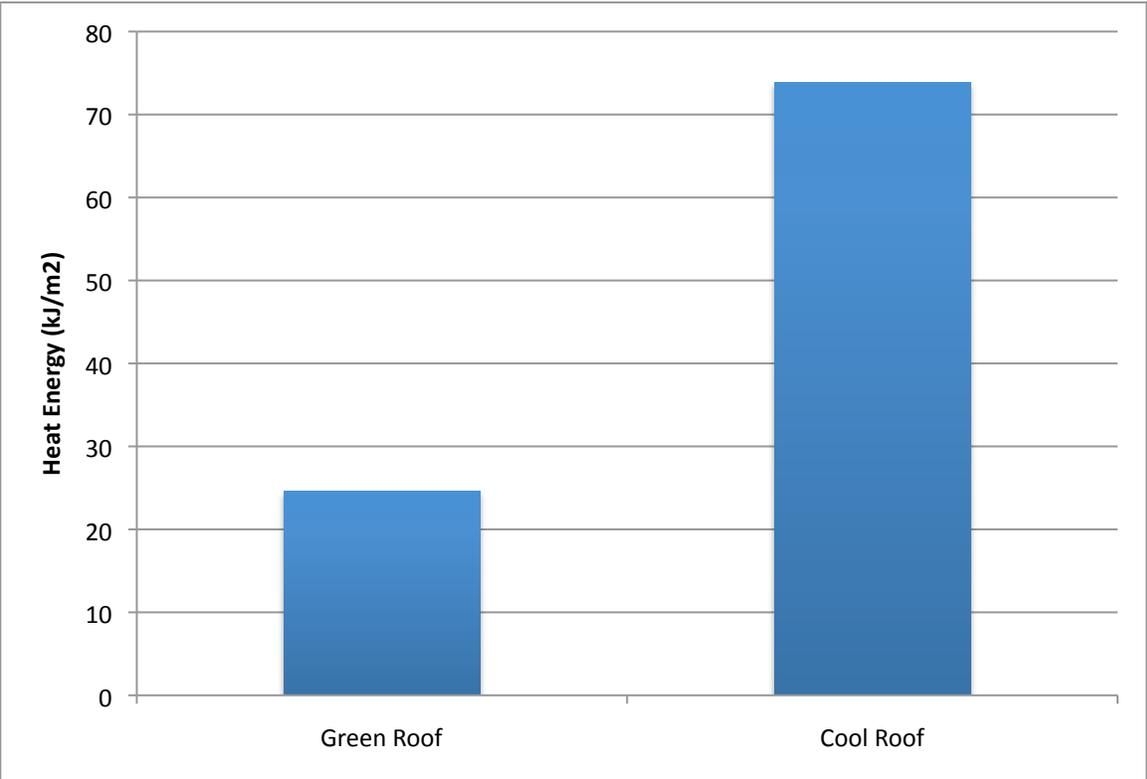
Figure 9: Roof Comparison, 12/03/2010
