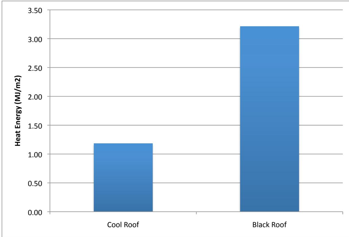
Figure 5: Roof Comparison, 10/22/2010 Data
