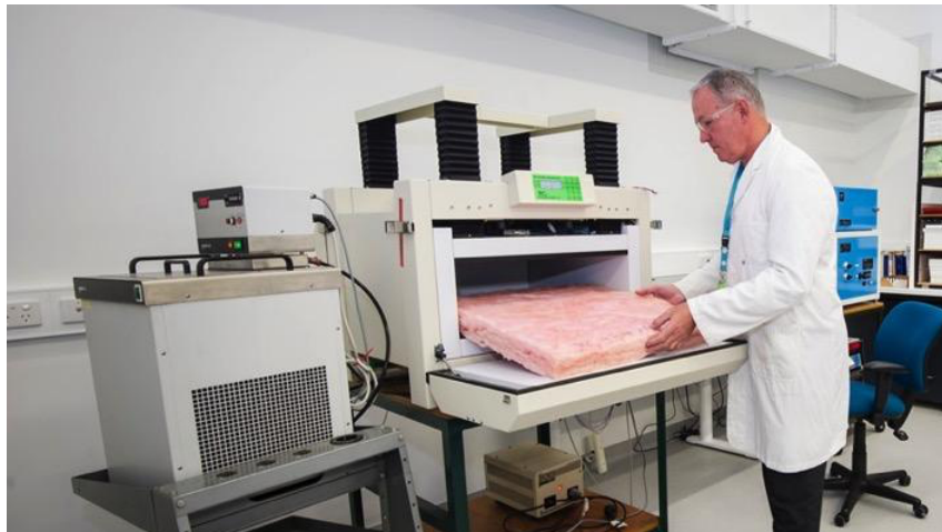
FIGURE 7: FIBREGLASS INSULATION TESTED TO LAB CONDITIONS OF 23°C, NOT REAL WORLD. CREDIT CSIRO [15]
