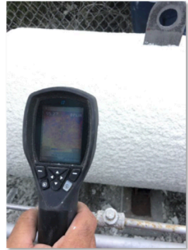
FIGURE 7: AIR IS COOLING THE UNPROTECTED SURFACE TEMP. ONCE CLOSED THICK FILM TIC IS APPLIED INCREASED SURFACE TEMPERATURE WITH ONLY PILOT HEAT WORKING
