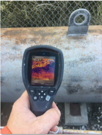
FIGURE 7: AIR IS COOLING THE UNPROTECTED SURFACE TEMP. ONCE CLOSED THICK FILM TIC IS APPLIED INCREASED SURFACE TEMPERATURE WITH ONLY PILOT HEAT WORKING
