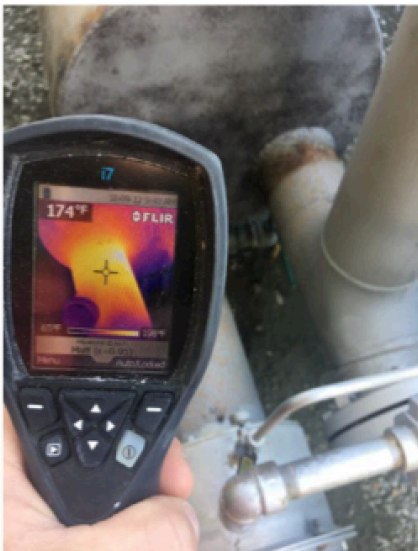
FIGURE 6: WATERBATH TEMPERATURE READINGS SHOWING 17C METAL TEMPERATURE IMPROVEMENT AFTER APPLICATION
