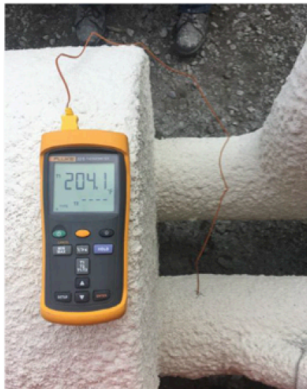
FIGURE 6: WATERBATH TEMPERATURE READINGS SHOWING 17C METAL TEMPERATURE IMPROVEMENT AFTER APPLICATION
