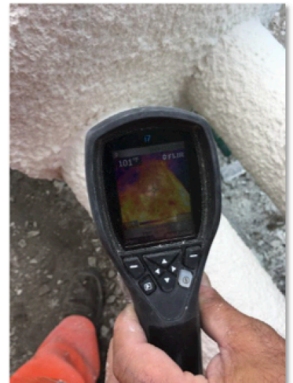
FIGURE 6: WATERBATH TEMPERATURE READINGS SHOWING 17C METAL TEMPERATURE IMPROVEMENT AFTER APPLICATION
