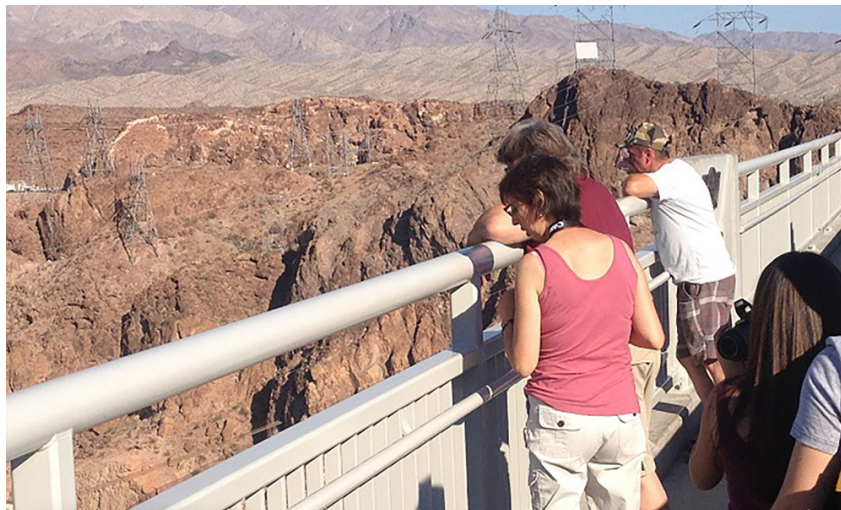
FIGURE 10: 3-5 MILLION PEOPLE HANDLING THE RAILINGS OF THE HOOVER DAM ENSURED THE CLOSED FILM THIN TIC REDUCED THE SURFACE TEMPERATURE ON THE RAILING FROM 63C DOWN TO 52.8C KEEPING VISITORS SAFE
